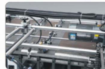
进口减速电机, 双张防冲顶装置 Imported speed-reducing motor, paper limit device
